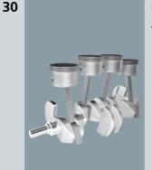
**Motor D 120 D** 12000 ccm, 176.5 kW, (240 PS), 17:1 **Vehicle** F 88, F 89, 1970-
